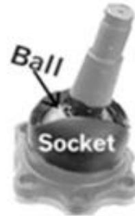
Figure 5.5 Universal Joint (Ball-and-socket)
